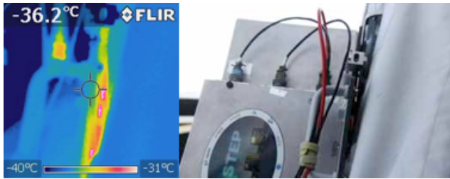
Fig. 16 Photographs of the ASTEP camera box at the interface with the telescope. Left: IR photograph showing the warm plume at the interface between the camera box and the telescope tube. Right: Visible photograph of the camera box and telescope tube.
